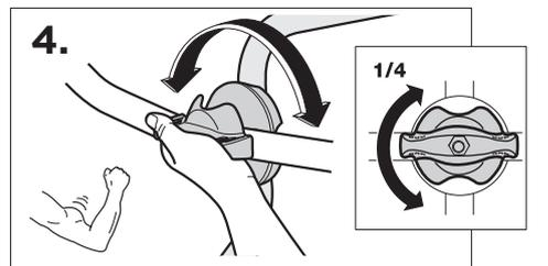
**EN** 1. Fit the knob as in the diagram. 2. Tighten the screw until it is no longer possible to undo the knob by hand. **3-4.** Loosen the screw 1/2 a turn at a time until it is possible to turn the knob by hand **(the knob should not move easily when it is loosened).**
