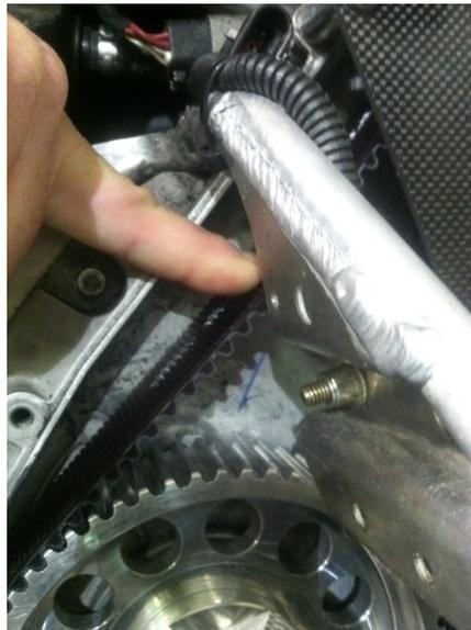
**Step 15:** Form the composite belt guard around the lip of the OEM chain case lip.
