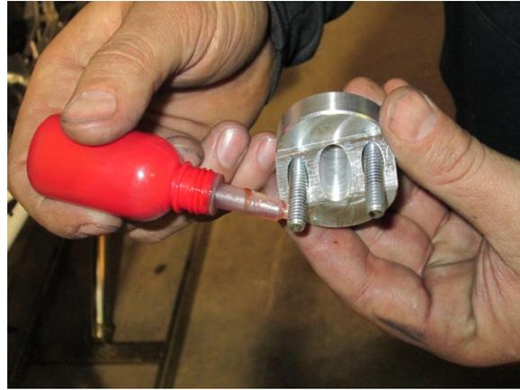
**Step 8:** Reinstall the ¼ - 20 bolts into lower pulley retainer finger tight. Install retainer assembly into lower driveshaft.
