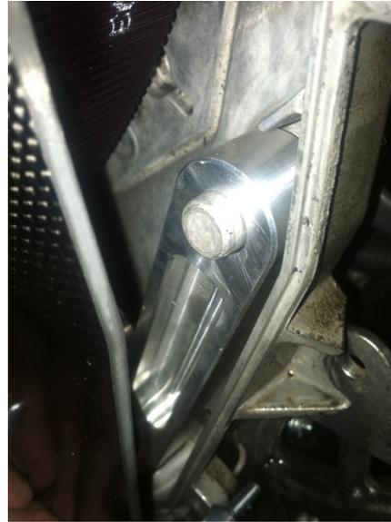
Step 11: Unlock Parking brake. Install upper pulley onto jackshaft, align belt cogs into pulleys, insert machined belt retaining flange into center bore of top pulley, and secure with OEM top gear retaining bolt and washer. Use Loc-tite on threads, and tighten to 30 ft/lb.
