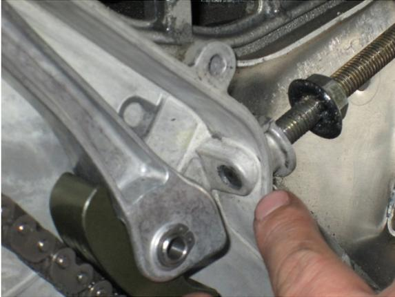
**Step 5:** Lock parking brake. Remove jackshaft gear retaining bolt (upper drive gear) using 15 or 16 mm socket. (Size depends on model year)
