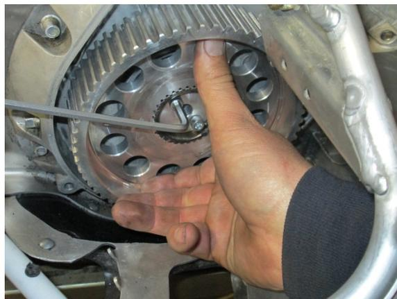
Step 13: Install speed sensor washer with included cap screw. Loc-tite cap screw center bolt, insert into lower pulley retainer, and tighten to 30 ft/lb.
