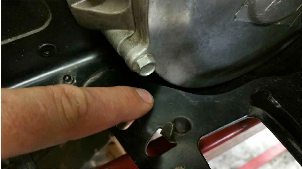
On T3 models this portion of the running boards needs to be trimmed or bent.
