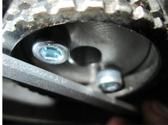
**Step 9:** Lower gear splines will fit tight you may need to heat center hub for gear to slide on or you may need to use a dead blow hammer to tap gear on. Slide new pulley onto lower driveshaft. Insert new drive belt through foot well, position onto lower pulley, and onto upper jackshaft.
