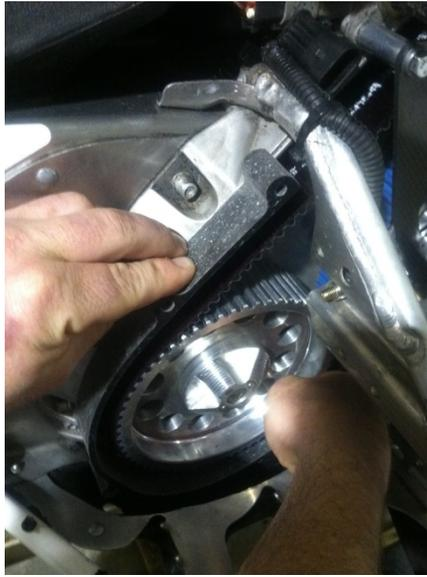
While holding composite belt guard in place, insert lower Carbon Fiber belt guard / speed sensor plate into position, and install retaining bolts.
