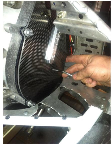
**Step 16:** Plug speed sensor into OEM sled harness, replace exhaust components, and hardware, and reinstall side cover.
