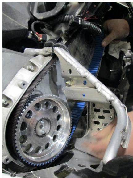
Step 10 : Install Carbon Fiber tensioner plate / tensioner assembly onto inner OEM chain case. Tensioner arm is installed onto OEM pivot boss. Loc-tite 3 bolts and tighten to 53 in/lb.
