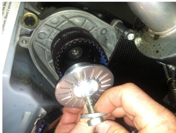
Step 12: Tighten lower driveshaft retainer cap screws to 16 ft/lb.
