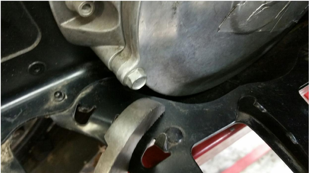
Use a large channel lock or like tool to roll the lip into the protective pan so bottom covers and gear will clear.
