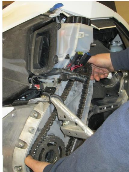
**Step 7:** Locate the new lower pulley retainer from the kit (photo below). Back the 2 pre-installed ¼ - 20 bolts out and apply 1 drop of blue Loc-tite to each bolt.
